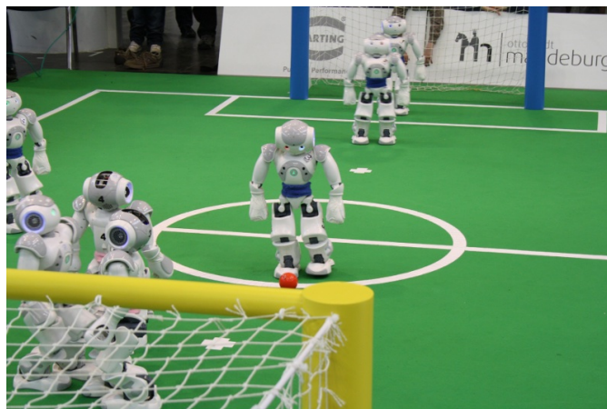
Fig. 1. RoboCup Soccer Standard Platform League: Nao robots autonomously playing a 4 on 4 soccer match in a color-coded environment.
